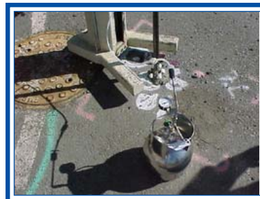
A Summa™ Canister is used to collect a soil gas sample near the storm water pipeline at Building 742.
