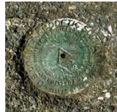
The U.S. Coast and Geodetic Survey from 1852 marks at the highest point on Mare Island Photo: Myrna Hayes
