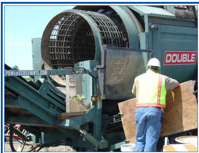
A Navy contractor monitors the progress of the soil screening near the clear, Lexan® shield used to protect workers.
