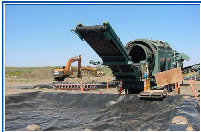
The rotating soil screen at the MCFR is shown here.
