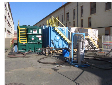
Water Filtration System for Removing Particulates from Water Generated during Cleaning and Flushing of IR14, the Industrial Wastewater Piping System
