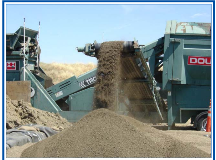
Dry screening for MEC from the historic outfall 4S using a Trommel
