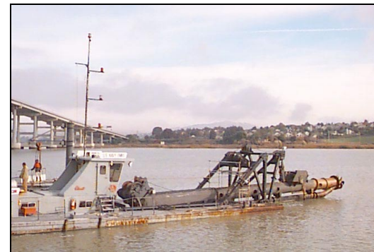
Floating Suction Dredge
