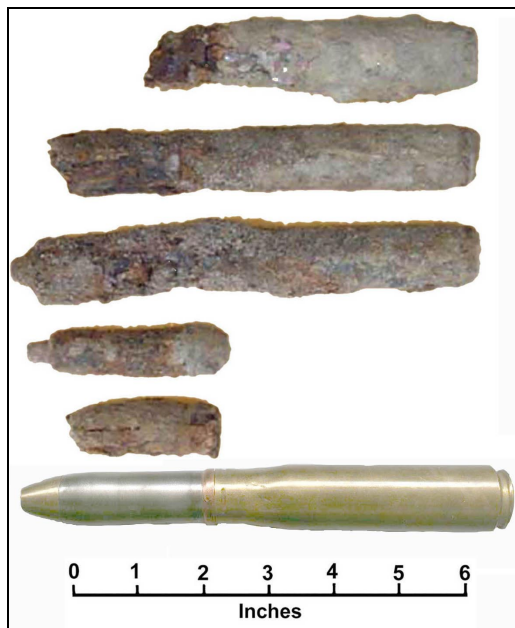
Comparison of New and Weathered 20 mm Ammunition
